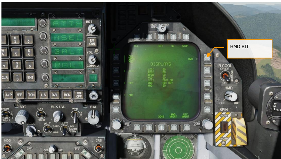
Figure 125. HMD Built in Test (BIT)
