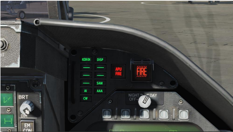
Figure 236. Right Instrument Panel Warning / Advisory / Threat Display Panel
