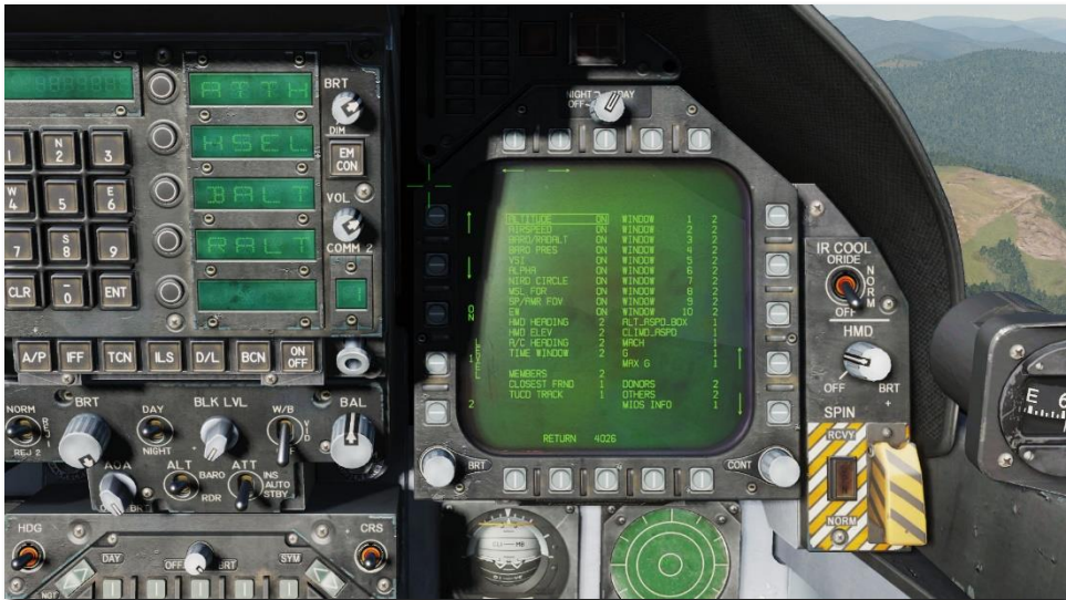
Figure 127. HMD Reject Setup Sub Level
