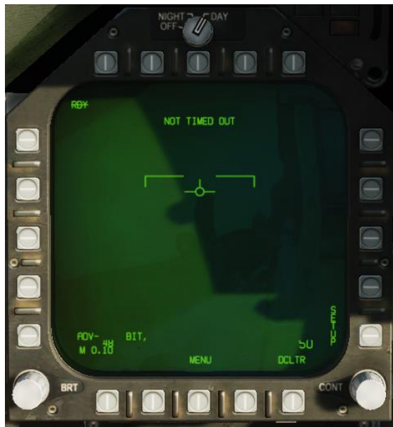
Figure 104. ATFLIR format in NOT READY mode.
