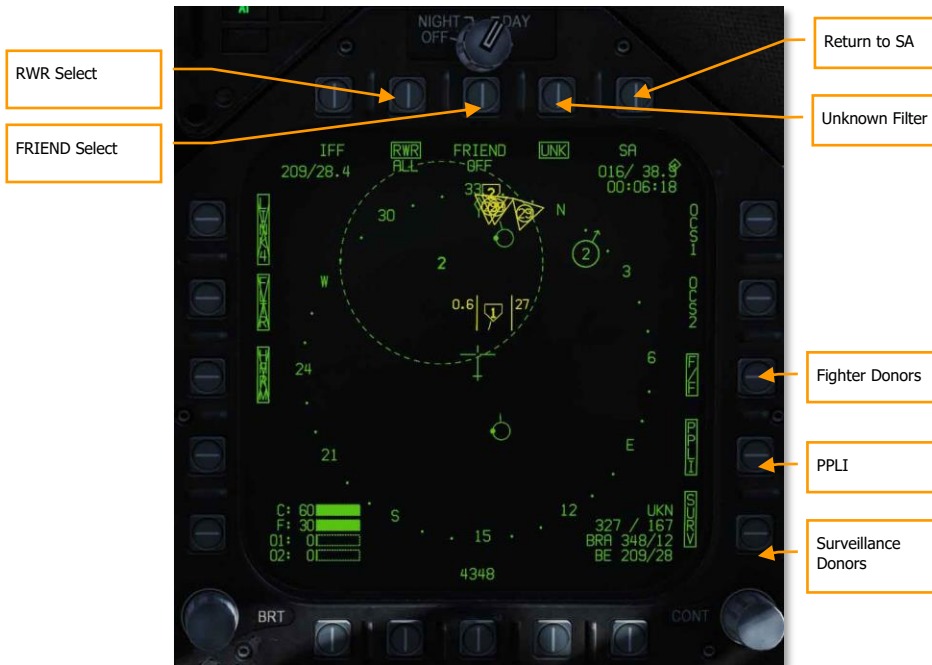
Figure 99. SA Page Sensors Sub-Level
