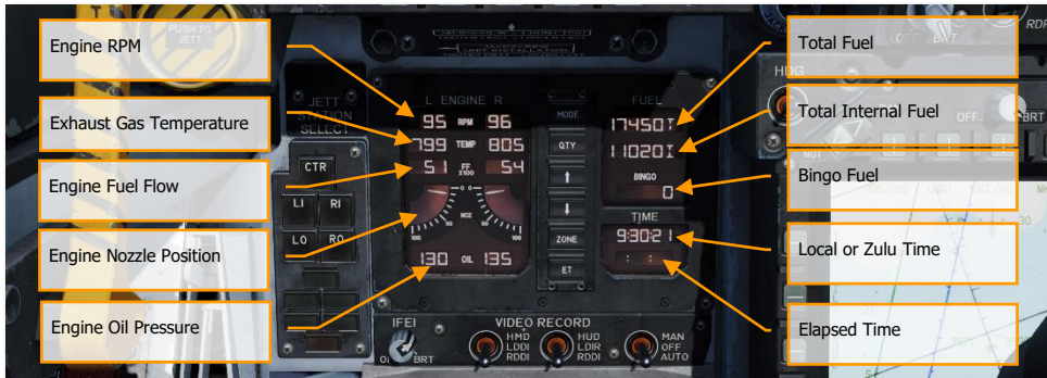
Figure 4. Integrated Fuel / Engine Indicator (IFEI)
