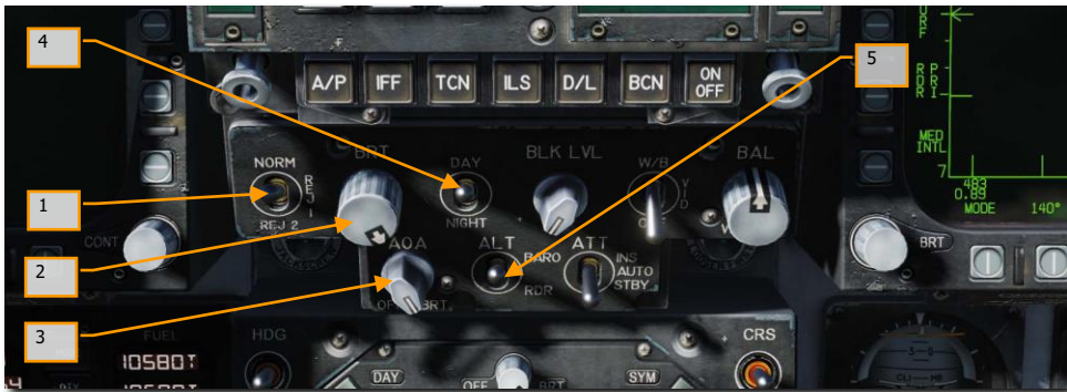
Figure 8. HUD Control Panel
